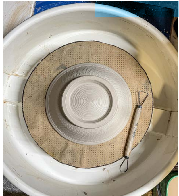
David brought along a piece of synthetic chamois, which when wetted sticks to the wheel head. A pot can then be placed on it for trimming or decorating. You could try a bat on it as well for throwing!
